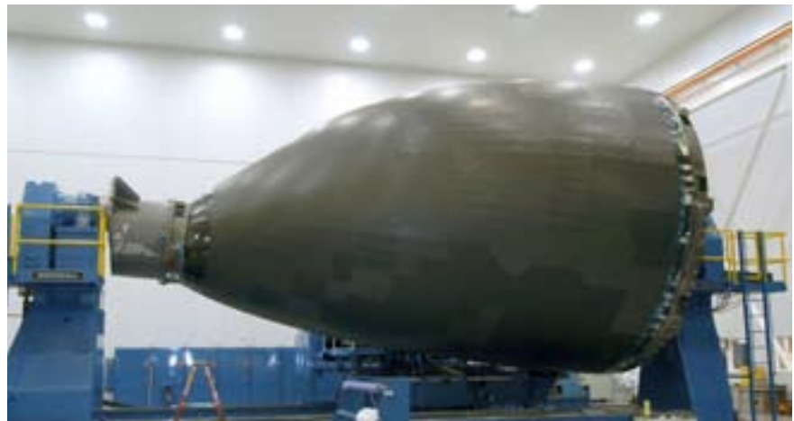
Fuselages are typically monolithic wound or tape laid structures with various thicknesses and may have complex curvatures, as in this B787 nose section. This constitutes a new level of challenge for composite repairers. (Picture © Boeing.)
