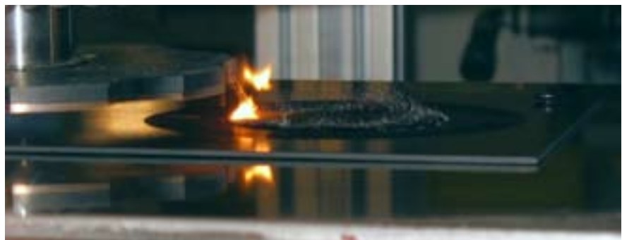
GKN Aerospace's prototype laser ablation machine used for repair site preparation.
