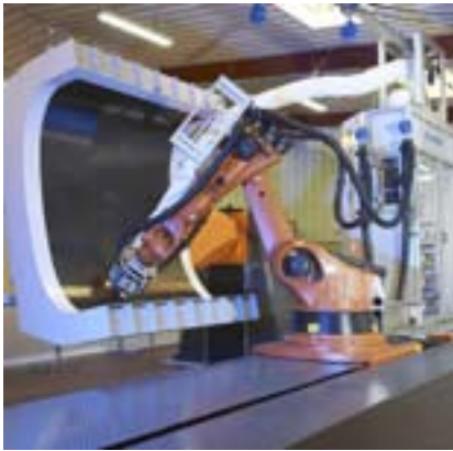
Multi-axis articulating robotic machines like this, currently being developed for manufacturing operations, could be adapted for automated repair use. (Picture courtesy of Coriolis Composites.)
