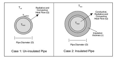
Figure 2.12 - Pipe Heat Loss
