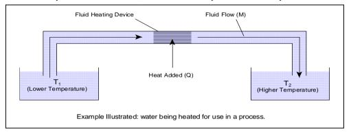
Figure 2.11 - Thermal Energy in a Hot or Cold Fluid
