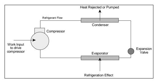
Figure 2.13 - Heat Flow in a Refrigeration System or Heat Pump
