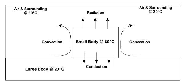
Figure 2.6: The Basic Heat Transfer Processes
