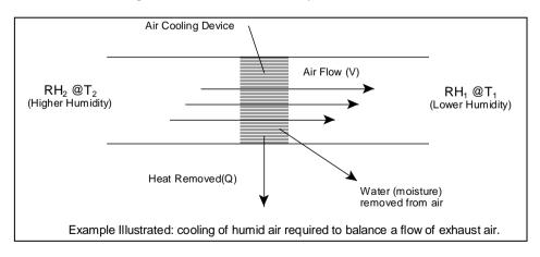
Figure 2.10 - Air Flow with Latent Heat
