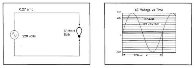
Figure 2.2: An AC Circuit and Waveform
