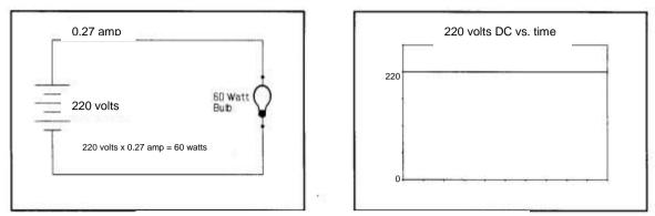
Figure 2.1: A DC Circuit and Waveform
