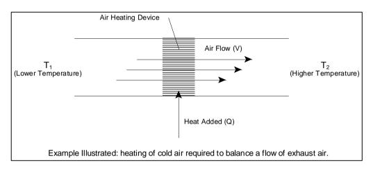
Figure 2.9: Air flow with sensible heat
