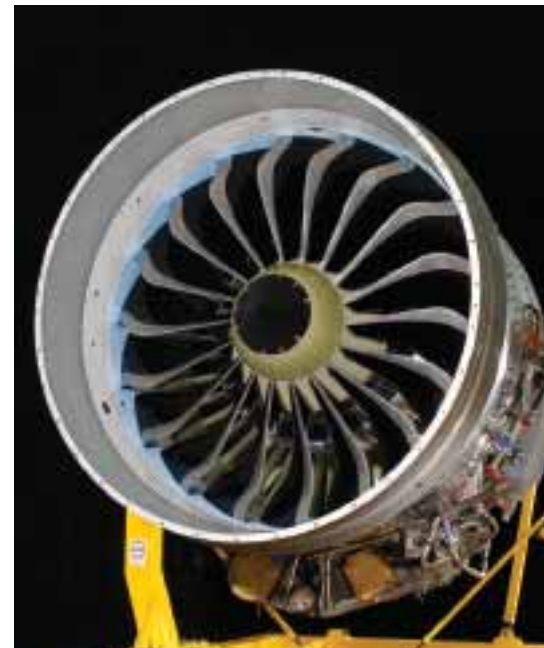
CFM's LEAP MASCOT demonstrator used a proprietary woven RTM process to knit CFRP material in three dimensions to create fan blades of the requisite size.
