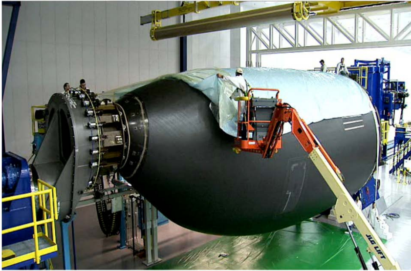
Composite Plane section fuselage Fire in London Boeing makes the 787's fuselage out of strands of carbon fiber layered around a rotating mold by a computer-controlled robot that looks like a spider. Boeing
