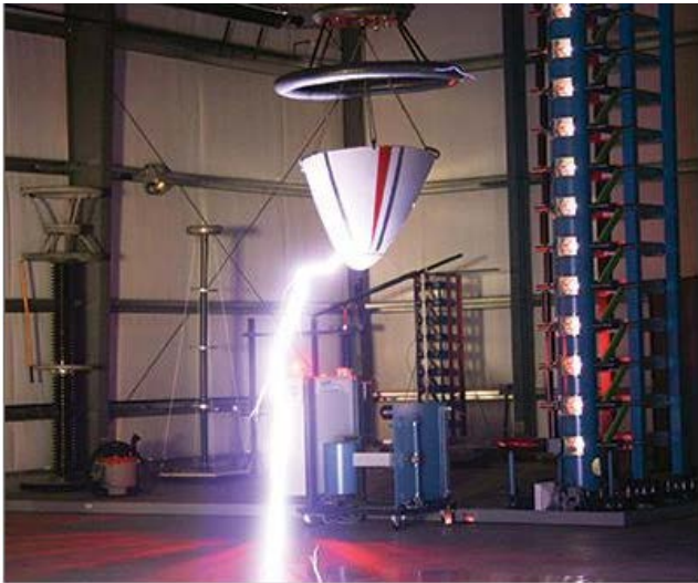
An aircraft radome undergoes lightning testing at National Technical Systems' (Calabasas, Calif.) lightning test laboratory. A 2.4-megavolt generator produces a strike to test the lightning strike protection (LSP) system on the part. Radomes are particularly susceptible to Zone 1A lightning, which can produce 200,000 amps. Source: National Technical Systems (formerly Lightning Technologies)
